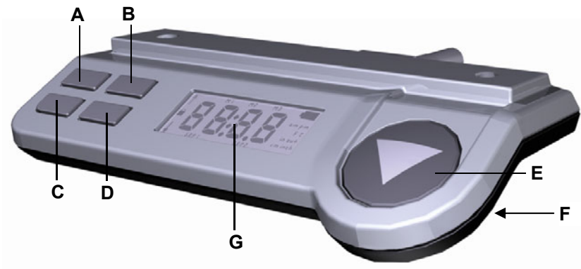
Figure 23 Motion Assist Pro control keypad function keys
