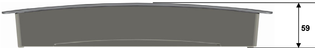
Figure 26 Dimensions of the Motion Manager 2 / 3 control unit, side view (in mm)
